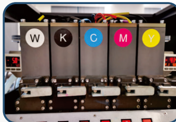
Negative Pressure System
